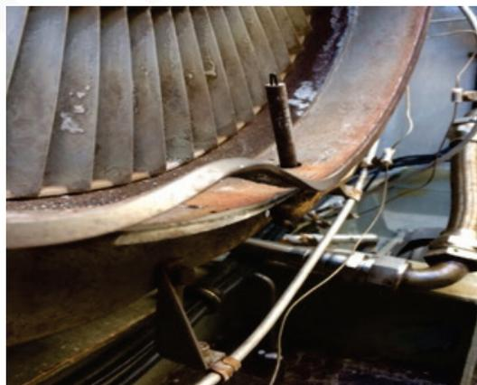
*Pictured: Damaged MPGT engine nozzle*
