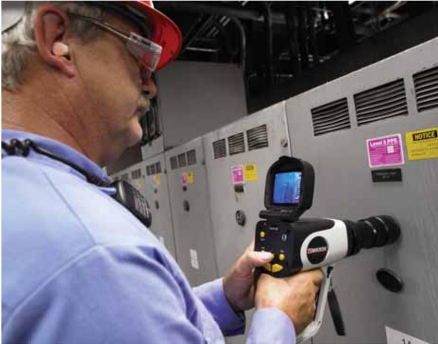
Maintenance technician Tom Anderson uses a Mikron camera equipped with a SpyGlass fish-eye lens to take infrared readings on an electrical cabinet.
