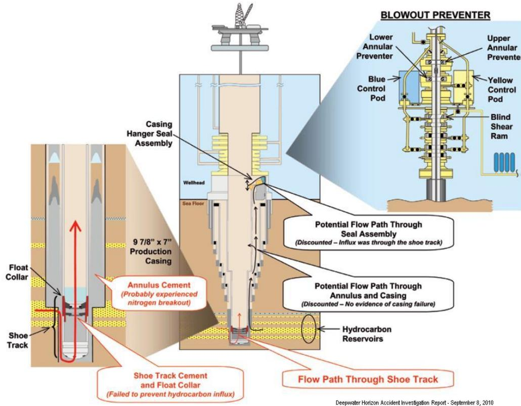
Figure 2. Illustration from the Deepwater Horizon Investigation Report.
